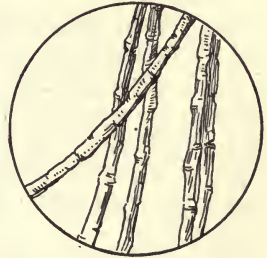
FIG. 58.—Linen fibers, showing the characteristic nodes and longitudinal striations.
